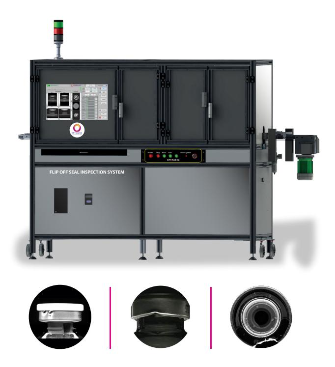
Optomech flip off seal inspection system is a high performance machine for checking the visual defects in a flip off seal
